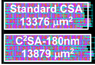
Fig. 3 Layouts of C 2 SA-180nm and standard CSA
