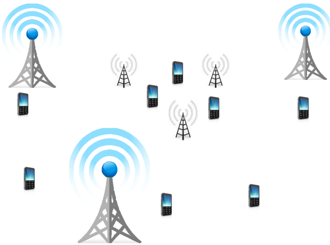
Fig. 1. HetNet is comprised of macro nodes and small nodes. Data traffic on the edge of macro cells are offloaded to the small cells, so that the performance on the macro-cell boundary area is improved and traffic load for the macro cell is alleviated.
