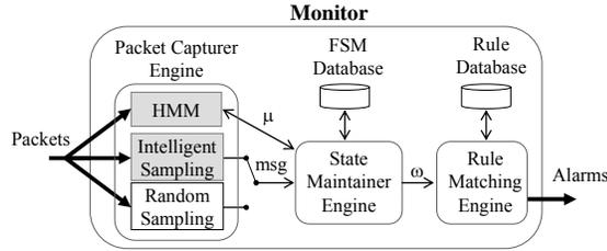
**Fig. 1.** Monitor architecture. One-sided and two-sided arrows show unidirectional and bidirectional flow of information respectively. Gray boxes indicate new components added to Monitor in this work.
