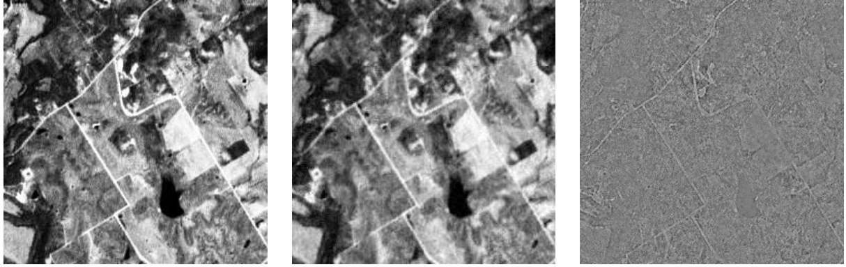
Fig. 2. With PCA basis: 2a: Original image 2b: Reconstruction using Compressive sensing 2c: Residue stored in database, with mean increased for clarity
