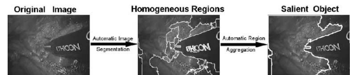
Fig. 2. Flowchart for our automatic salient object detection function, where the neighboring images regions with the same semantic label are automatically aggregated to form a certain type of the concept-sensitive salient objects.
