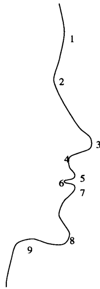
Fig. 12. The nine fiducial points of interest for face recognition using profile images (similar to figure in [61]).
