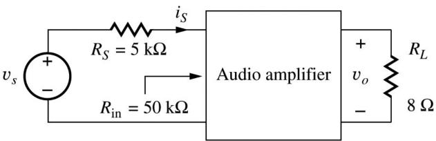
7) Which one of the current gain  $(A_i)$  frequency response curves belong to the amplifier shown below?
