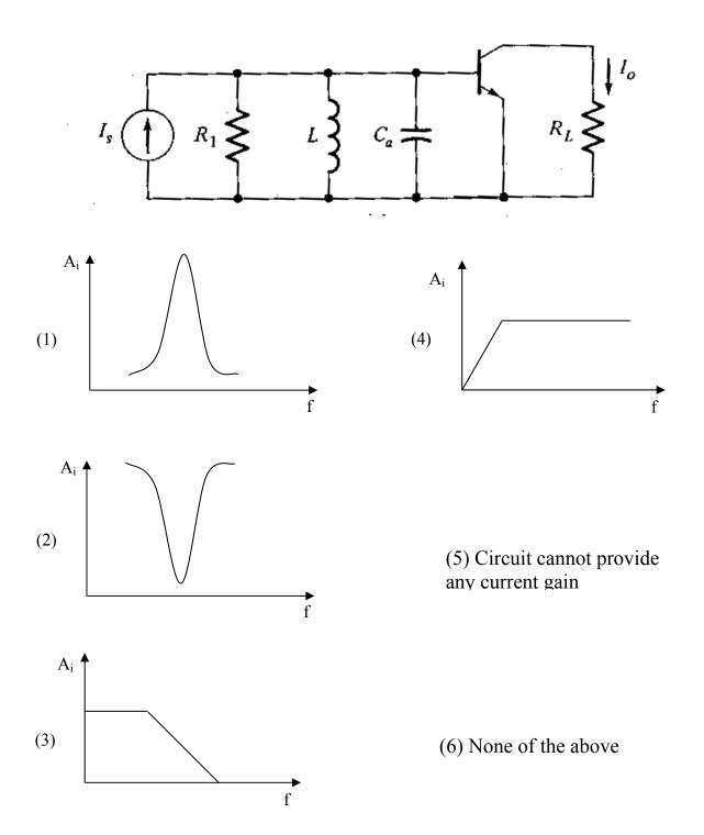
18. For the amplifier circuit shown below estimated value of  $f_L$  is? For BJT assume  $\beta$ =150,  $V_A$ =75V,  $V_{BE}$ (on)=0.7,  $V_T$ =25 mV.
