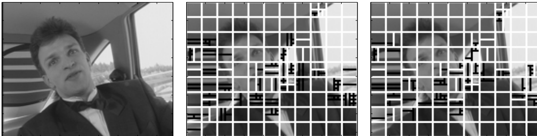
Fig. 6. A frame of the Carphone sequence (left) and its two tilings: dyadic transform tiling with H.264/AVC motion compensation tiling (center) and multitree transform tiling with H.264/AVC motion compensation tiling (right). The motion compensation tiling and transform tiling are indicated with white and black lines, respectively.
