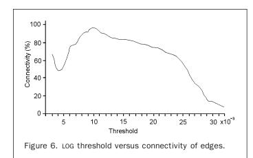
the final edge image. In this example, the final determined LOG threshold is  $T_{LoG} = 0.01$ , which leads to a connectivity of 94 percent.
