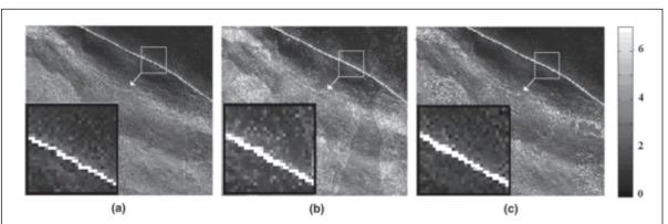
Figure 4. Slopes calculated with different methods: (a) finite difference, (b) D8, and (c) weighted average.
