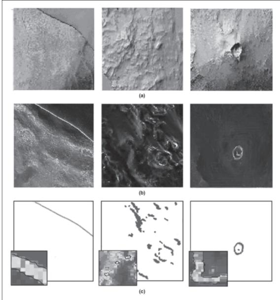
Figure 11. (a) shaded relief images, (b) slope maps (brighter pixels for higher slope), and (c) extracted features.
