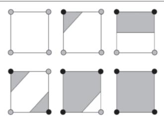
Figure 8. Distinct cases for marching square algorithm (dark dot: inside feature cell; light dot: outside feature cell; shaded area: feature interior).
