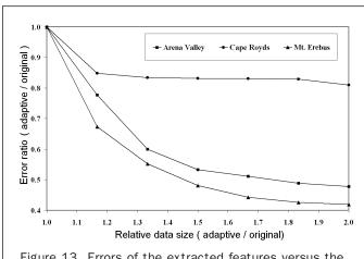
Figure 13. Errors of the extracted features versus the number of shoulder points in the adaptive method.
