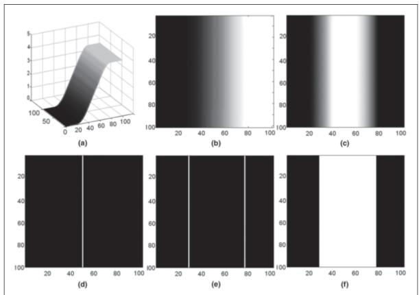
Figure 2. Edge detection: (a) hyperbolic slope surface, (b) DTM, (c) slope map, (d) LOG of DTM, (e) LOG of slope map, and (f) feature with simple edge (white).
