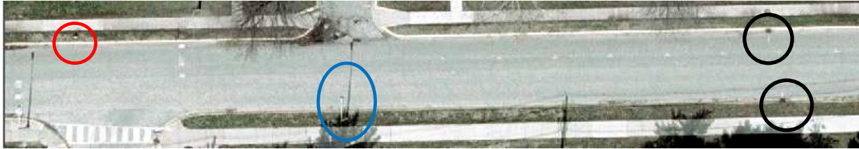
Figure 2. 7.5cm aerial image showing storm water inlets (black), electric pole (blue) and fire hydrant (red).
