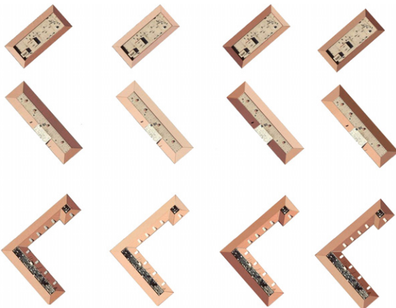
Fig. 6. Shade correction of roof images, 1st column: Original texture image at sun direction ( A_s: 161.75^\circ, Z: 46.82^\circ ); 2nd column: Shade-free texture image; 3rd column: Texture rendering at sun location ( A_s: 341.75^\circ, Z: 46.82^\circ ; opposite to the 1st column); 4th column: Texture rendering at the same sun direction as the original image. North is to the right.
