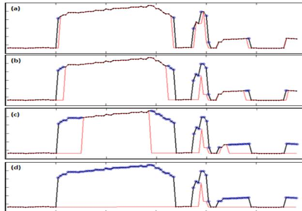
**Figure 1.** Filtering of a LiDAR profile, (a)-(d) Intermediate plots of different iteration steps, (black dots) lidar points, (blue dots) filtered nonground points and (red line) morphologically eroded surface.
