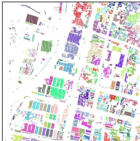
**Figure 3.** Separated individual building points
