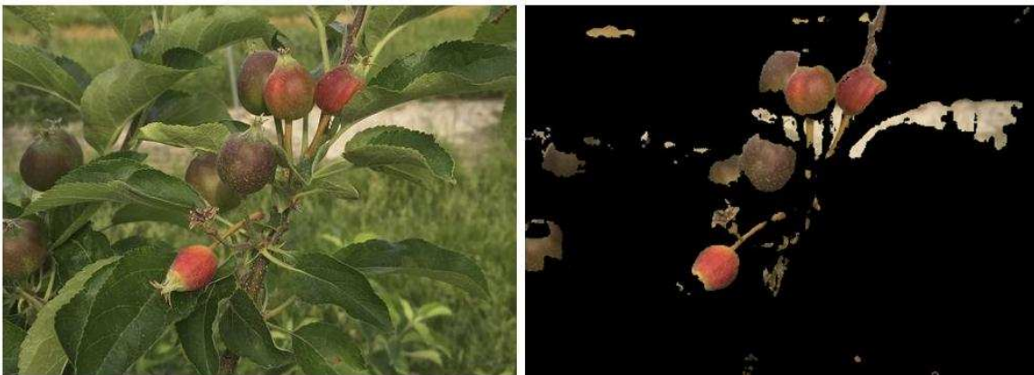
Figure 10: The goal here is to segment out the fruitlets from the image on the left. The segmentation shown at right is based on just hue filtering. We accept all pixels whose hue values are between 0^\circ and 30^\circ . The image at left was supplied by Dr. Peter Hirst, Professor of Horticulture, Purdue University. The segmentation result shown was obtained by invoking the function apply_color_filter_hsv() of my Python based Watershed module.
