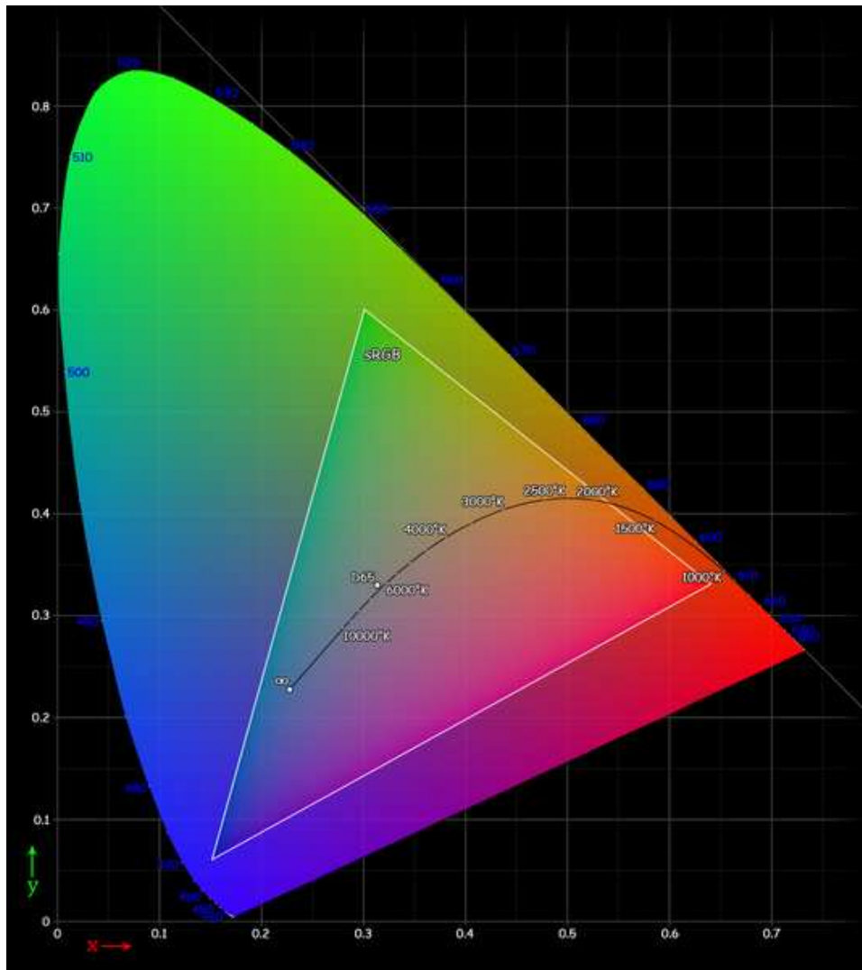
Figure 17: Projection of the Chromaticity Plane on the XY-plane gives us the Chromaticity Diagram. The triangle in the middle is the sRGB color gamut that most electronic displays are capable of displaying. The larger rounded cone is what the human eye can see. The colors on the periphery of the large rounded cone are the spectral colors. As you change the wavelength of a monochromatic light beam over the entire spectral range visible to humans, you will move along the rounded perimeter shown in the diagram. The arc in the middle shows what is known as the Planckian Locus. The numbers shown along the arc are the temperatures to which you must raise an incandescent black body for it to emit the light at that point in the diagram.
