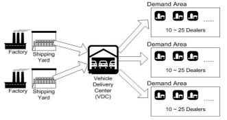
Figure 1: One VDC with two "parallel" shipping yards.
