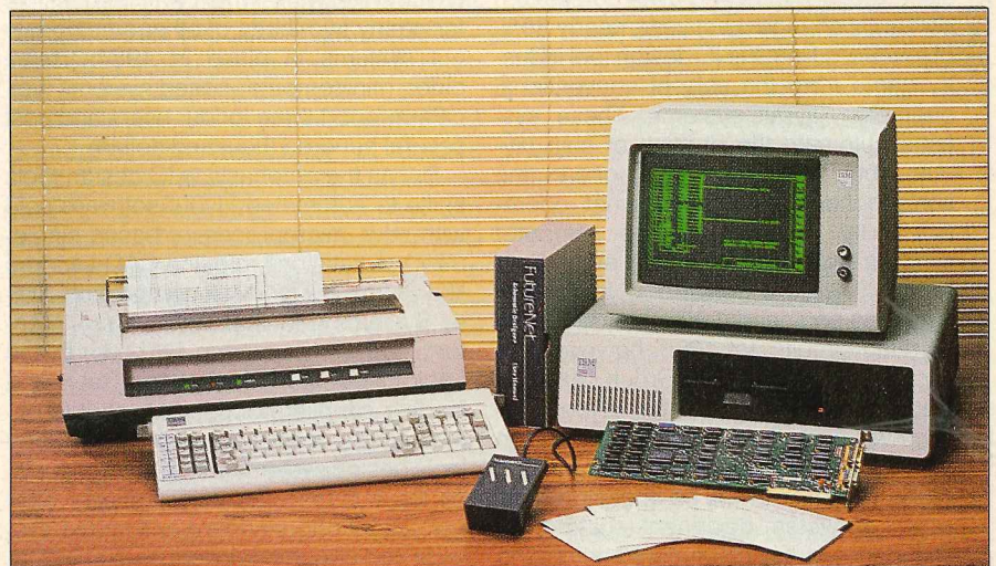
Plug-in special-purpose processors, such as this system developed by FutureNet, turn the IBM PC into an engineering workstation that can handle many aspects of integrated circuit design.
