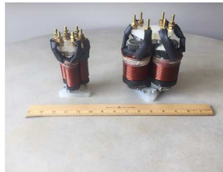
Utility-side and inverter-side 3-phase ac inductors for 1 kV 50 kVA PV inverter
