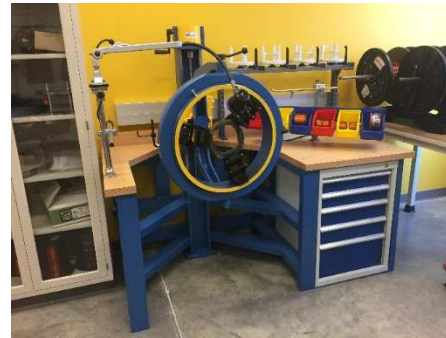
Stator assembly station
