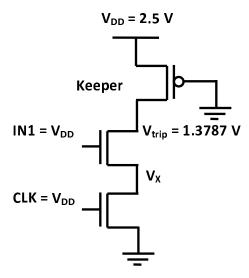
With the values of the threshold voltages provided, all the transistors are in **linear** region. Equating the current through the PDN NMOS and the evaluate NMOS, we get
