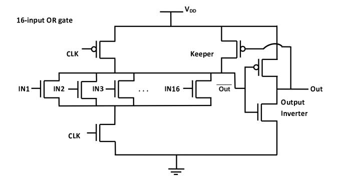
**Part a):** Determine (by hand calculation) the width of the keeper PMOS ensuring the *correct functionality* of the gate. You can select the characteristics of the output inverter by your own *with explanation*. State your assumptions, if any. Use the following information.
