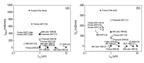
Fig. 3. Historical comparison of published dc (a) maximum drain current  $I_{MAX}$  and (b) transconductance  $G_m$  of n-channel E-mode III–V MOSFETs from 1965 until today.
