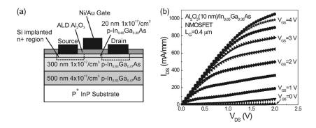
Fig. 1. (a) Cross section of an inversion-type E-mode  $Al_2O_3/In_{0.65}Ga_{0.35}As$  MOSFET. (b) I-V characteristic of a 0.4- $\mu$ m gate-length  $In_{0.65}Ga_{0.35}As$  MOSFET with a 10-nm ALD  $Al_2O_3$  as gate dielectric.
