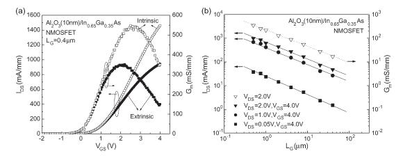
Fig. 2. (a) Extrinsic and intrinsic drain current and transconductance versus gate bias at  $V_{\rm DS} = 2.0$  V. (b) Extrinsic drain current at  $V_{\rm GS} = 4.0$  V and  $V_{\rm DS} = 2.0$  V,  $V_{\rm DS} = 1.0$  V, or  $V_{\rm DS} = 0.05$  V versus  $L_G$  and the extrinsic peak  $G_m$  at  $V_{\rm DS} = 2.0$  V versus  $L_G$ . The solid and dotted lines are guided by eyes.
