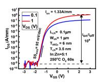
Fig. 14.  $I_{DS}$ -V<sub>GS</sub> transfer characteristics of an annealed InZnO (In: Zn=5:1), exhibiting SS of 95 mV/dec, and 1.33 A/mm on-current.
