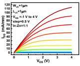
Fig. 7. Output curves of a long-channel InZnO (1:1) transistors with  $L_{ch}$ =1  $\mu$ m and  $W_{ch}$ =1  $\mu$ m before O<sub>2</sub> annealing showing well-behaved DC characteristics and current saturation at high V<sub>DS</sub>.
