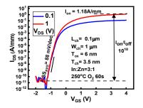
Fig. 13.  $I_{DS}$ - $V_{GS}$  transfer characteristics of an annealed InZnO (In: Zn=3:1), exhibiting SS of 88 mV/dec, and 1.18 A/mm on-current.
