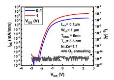
Fig. 10.  $I_{\rm DS}\text{-}V_{\rm GS}$  transfer curves of the same device as in Fig. 9.
