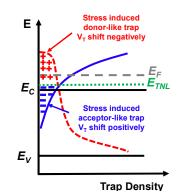
Fig. 19. Model of  $V_T$  shifts under PBS on InZnO FETs. This is the key understanding of this work.
