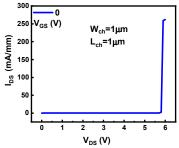
Fig. 22. Off-state breakdown measurement of InZnO transistor (In: Zn=1:1) limited by the ultrathin dielectric and the depleted InZnO layer.
