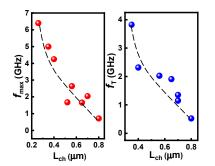
Fig. 23. Channel-length dependence of  $f_T$  and  $f_{max}$
