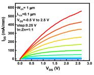
Fig. 12.  $I_{DS}\text{-}V_{DS}$  output characteristics of the same device in Fig.11 after  $O_2$  annealing. Similar  $I_{on}$  can be achieved at higher  $V_{GS}$  and  $V_{DS}$ .
