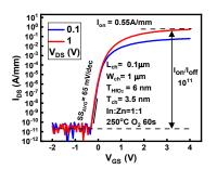
Fig. 11.  $I_{DS}$ -V<sub>GS</sub> transfer characteristics of an annealed InZnO (In: Zn=1:1) transistor of Figs. 9-10, exhibiting better SS of 65 mV/dec and  $I_{on}/I_{off}$  ratio, and similar 0.55 A/mm as on-current  $I_{on}$ .
