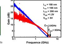
Fig. 21. Unilateral gain and  $h_{21}$  from a 0.35µm channel length InZnO RF transistor (In: Zn=5:1).
