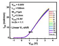
Fig. 16.  $I_{DS}$  vs.  $V_{GS}$  relationship with stress time up to 1500 s for a large positive gate bias stress.
