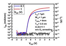
Fig. 8. Transfer curves of the same device in Fig. 7, showing low gate leakage current and also well-controlled off-state performance.
