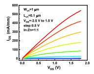
Fig. 9.  $I_{DS}$ -V<sub>DS</sub> output curves of a shortchannel InZnO (1:1) transistor with  $L_{ch}$ =0.1  $\mu$ m and W<sub>ch</sub>=1  $\mu$ m before O<sub>2</sub> annealing.
