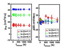
Fig. 17.  $\mu_{FE}$  and  $\Delta SS$  dependence on stress time with gate biased at  $V_T$  +3V. Each data point represents the average of at least five devices.
