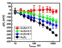
Fig. 18.  $V_T$  shifts negatively with stress time increasing in different In:Zn ratios in the statistical measurement, with gate biased at  $V_T$  +3V. Negligible  $V_T$  shift is obtained for 1:1 InZnO. Each data point represents the average of at least five devices.
