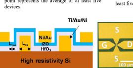
Fig. 20. Schematic and optical microscope image of RF circuits with GSG (ground-signal-ground) structure. In:Zn=5:1 film is employed for better contact and higher  $g_m$ . Highly resistive intrinsic silicon (>10 k $\Omega/\Box$ ) is selected to reduce the substrate parasitics.
