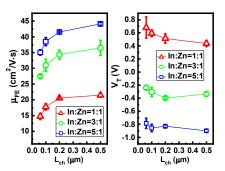
Fig. 15. Statistic results of channel-length dependent field-effect mobility and threshold voltage with different In:Zn ratios (each data point represents the average of at least five devices).
