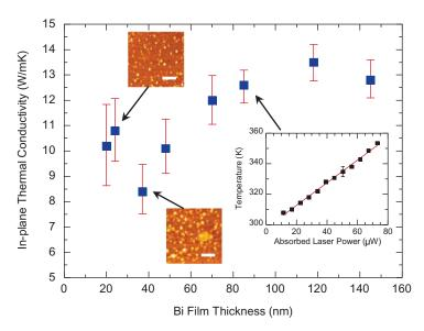
**Figure 3** In-plane thermal conductivity of Bi films. The inset plots the measured temperature vs. absorbed laser power for the 85-nm film, and the black solid line is a linear fit. The inset pictures are atomic force microscope images of the 24- and 37-nm film surfaces, which show different surface feature densities. The scale bars are all 1  $\mu$ m.
