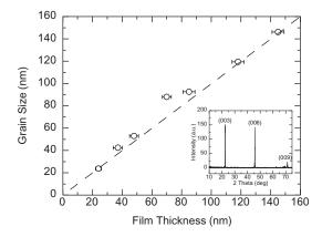
Figure 4 Grain sizes of Bi films calculated from the (003) peak of the X-ray diffraction data using Eq. (9). Grain size uncertainty is  $\sim$ 1 nm. The dashed line corresponds to where the grain size equals the film thickness. The inset shows a typical X-ray diffraction pattern. The angle step size is 0.02°.
