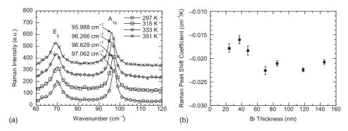
Figure 2 (a) Raman spectra taken under different temperatures during the calibration of 85-nm-thick Bi sample. Data are shifted vertically for a clearer view. The inset numbers denote the Lorentz fitted peak position of the  $A_{1g}$  Raman mode. (b) Calibration results of Raman peak shift vs. temperature.
