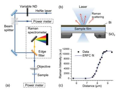
Figure 1 (a) Schematic of the experimental setup. (b) Schematic of the sample structure. The sample film is sandwiched between the Raman sensor Bi and the substrate  $SiO_2$ . The film stack lies on an Si frame. For the measurement of Bi films, there is no layer in between. (c) Laser spot size measurement results. The blue curve is the complementary error function fitting of the data.
