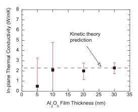
Figure 5 In-plane thermal conductivity of Al<sub>2</sub>O<sub>3</sub> films. The dashed line corresponds to the kinetic theory prediction by Eq. (10) under the assumption that the phonon mean free path is restricted to be equal to the interatomic distance in amorphous solids.
